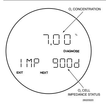
Figure 3-23. CELL IMPEDANCE
